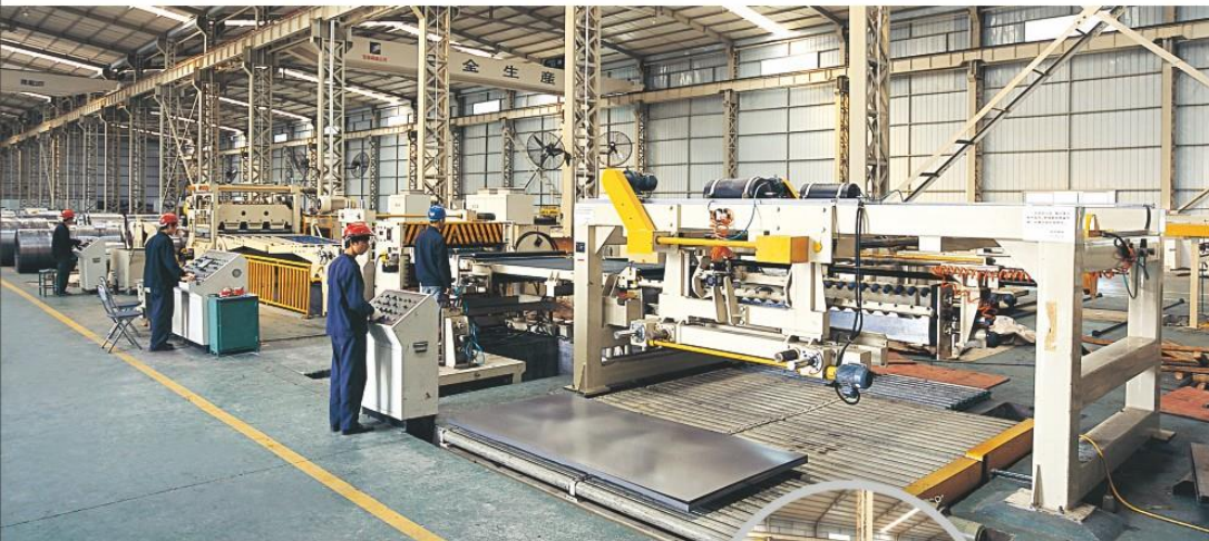
大型自動平整板裁切機 Automatic flatbed panel tailoring and cutting unit
